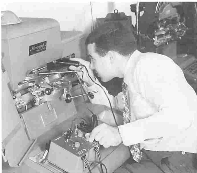
Figure 3-2. Using the Stroboslave to illuminate the interior of a metal stencil imprinter.
