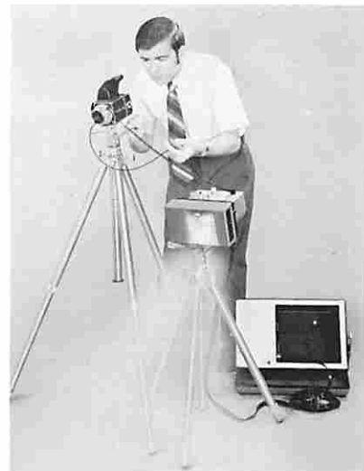
The Strobolume is ideal for synchronized, single-flash high-speed photography—even in color. For example, the 1540 has a guide number of 70 when used with High-Speed Ektachrome (ASA 160).
